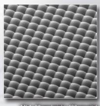
MLA, 20 µm height, 100 µm pitch
