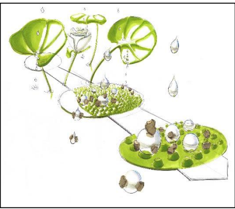
Artist impression of self-cleaning and colour properties that can be created through injection moulding in polymer surfaces. Functionalities are inspired from nature, but the structures are designed for manufacturing.
