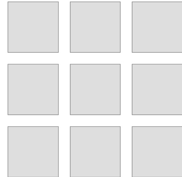
Each of the patterned fields are composed of 1 mm x 1 mm areas with line gratings with the specific lateral dimension and spacing. The 1 mm x 1 mm areas are arranged in a 3 x 3 array with 100 \mu\text{m} spacing.
